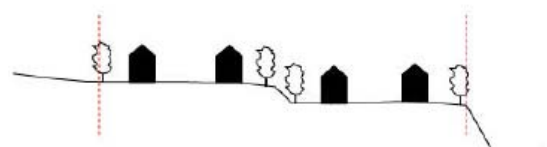
Figure 25: Section BB showing an indicative option for retaining an embankment within the centre of the site to tackle the gradient change
