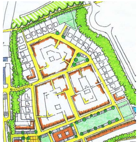
Suggested development framework with single plot depth on periphery and perimeter blocks in middle
