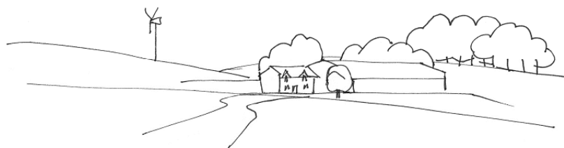
Image 1: A turbine illustrated at an indicative 2x height of the house from this view, or a taller turbine located behind the ridge to reduce overall height from this view. The turbine is well scaled in relation to the size of other individual features. It is also located on the side of the hill, rather than the hill top, where it can be 'read' in conjunction with the farm buildings. This forms a 'cluster' of development, which reduces landscape and visual impact.
